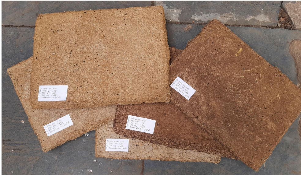
Fig 30: Biomass Panels having different compositions of crop residues and fibres as explained above.
