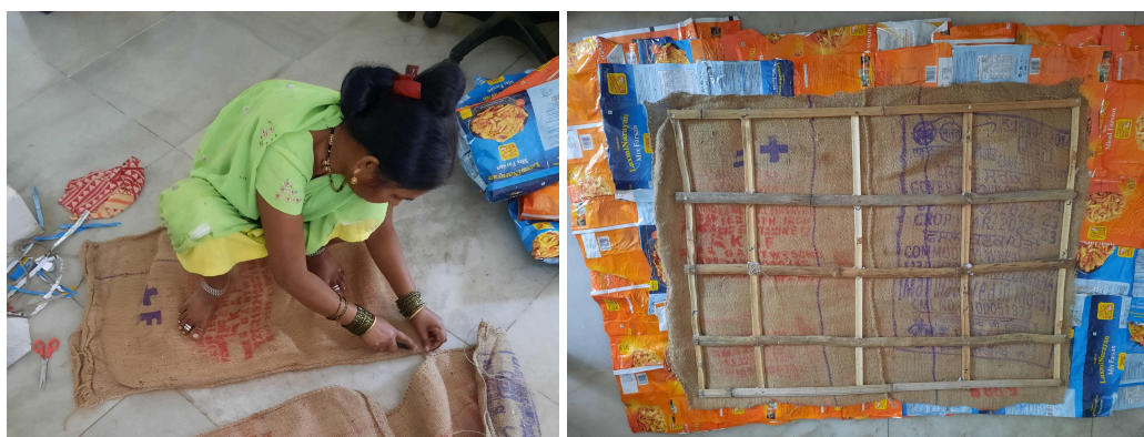
Fig 26: Assembling Jute and MLP Sheets on Bamboo Frame
