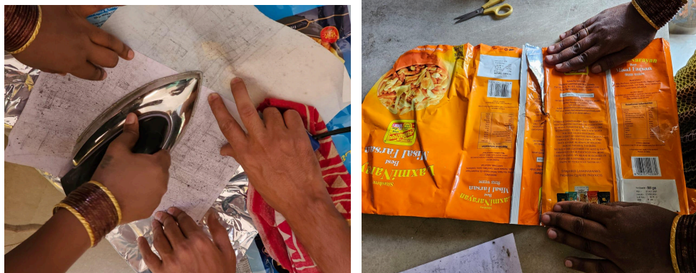
Fig 25: Joining MLP Wrappers to form 3x4 feet sheet
