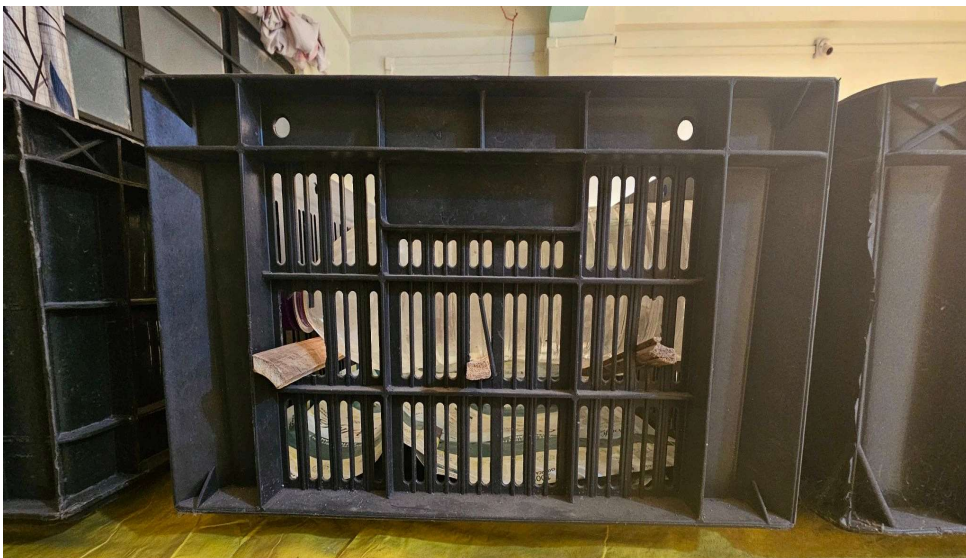
Fig 35.1.1-12 : Crate with Elevated Bamboo Base (Side View)
