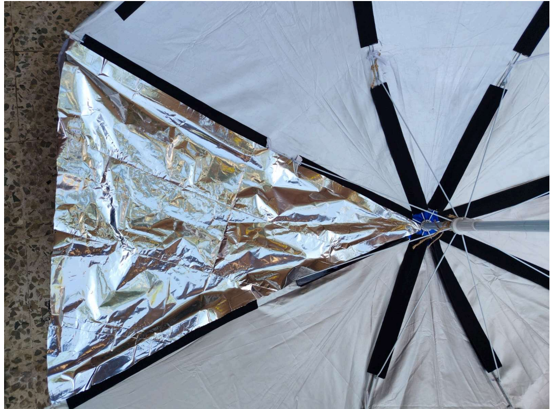
Fig 35.8.1-12 : MLP Sheets Pressed to the Umbrella
