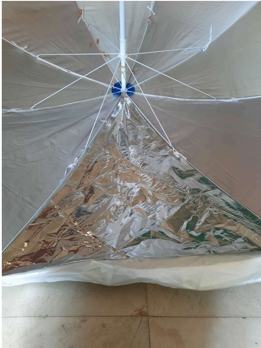
Fig 35.8.1-8 : Triangular Panels Attached to Umbrella Underside
