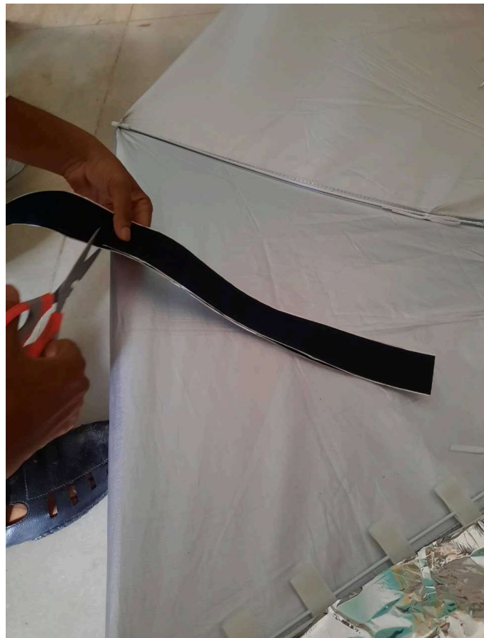
Fig 37.9.2.1.1-1 : Measuring & Cutting the velcro strip to the exact length of the spoke
