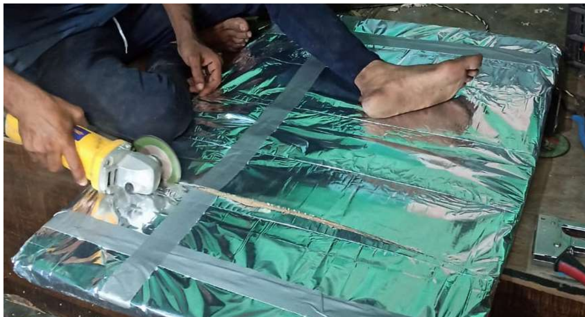
Fig 37.2.5-5 : Cut the whole panel
