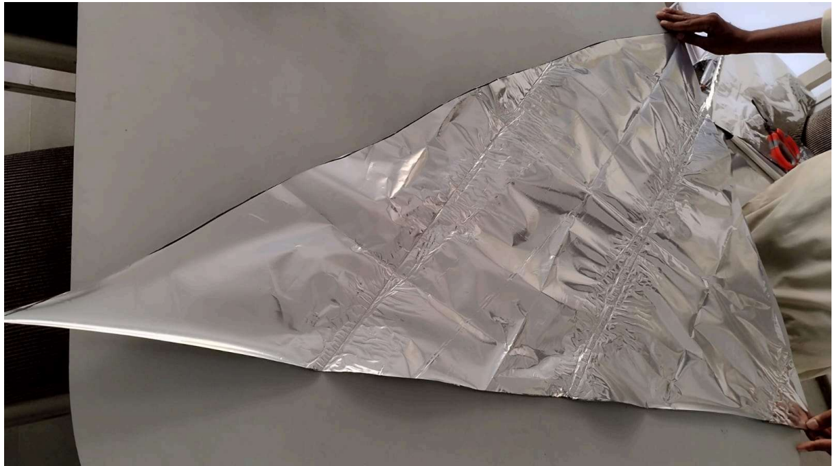
Fig 35.8.1-1 : Cutting of MLP Sheets into Triangular Shapes
