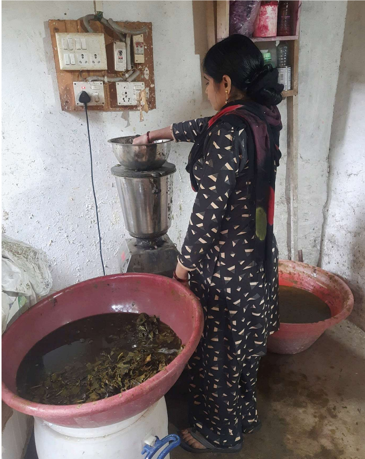
Fig 37.2.2-9 : Grind the boiled fibres to a pulp in an industrial mixer
