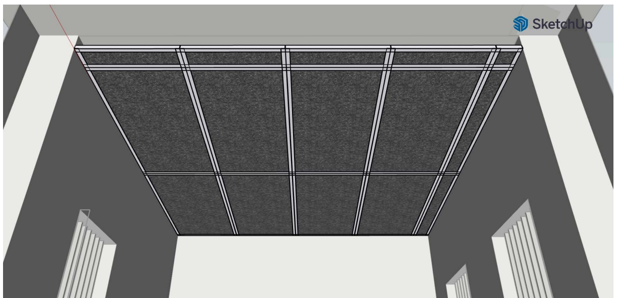
Fig 37.3.2-4 : Metal support framework with panels in place
