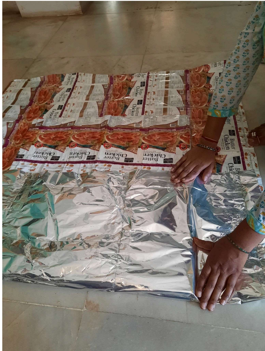
Fig 37.8.2.1.5-1 : Positioning MLP Layer of size 3feet x 4 feet at the bottom for wrapping the assembly.
