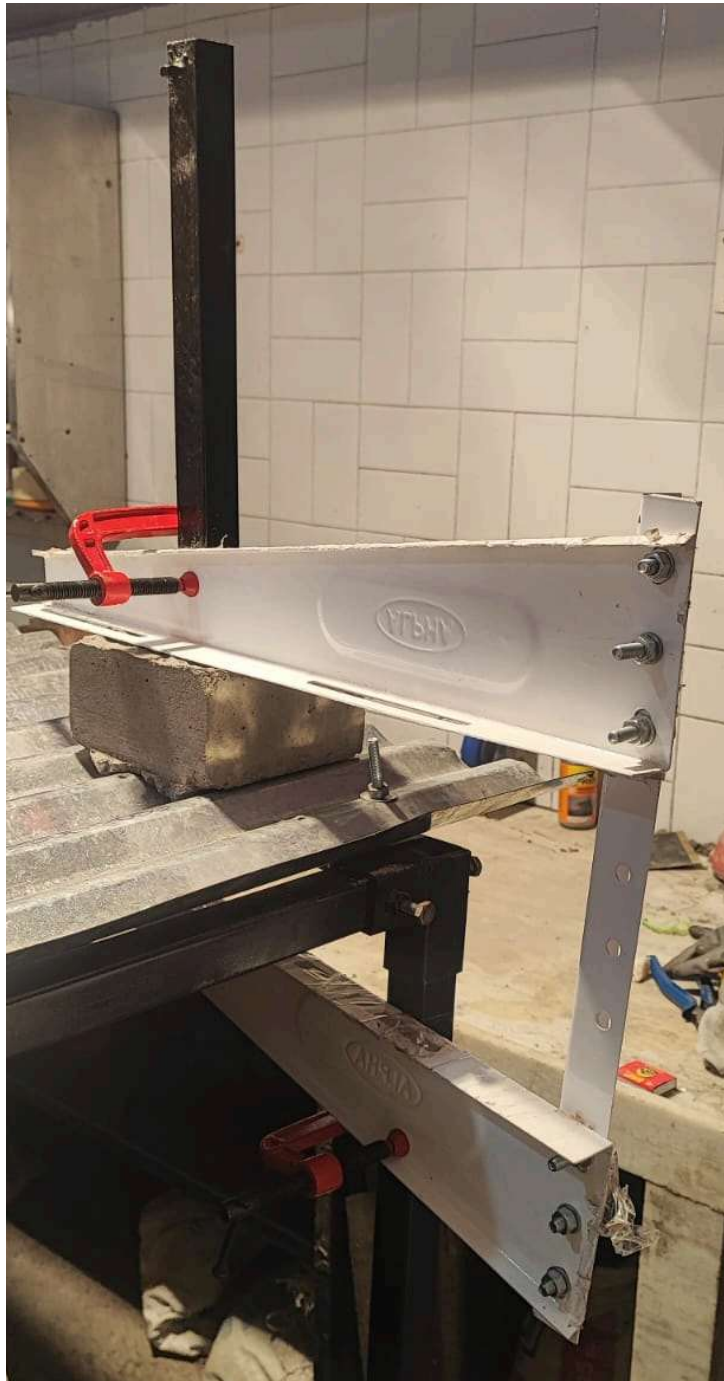
Fig 35.2.1-2 : Prototyping the Clamp-Based Support for Space Frame
