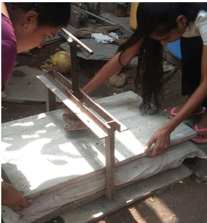
Fig 37.2.2-11: Press the panels to remove excess water
