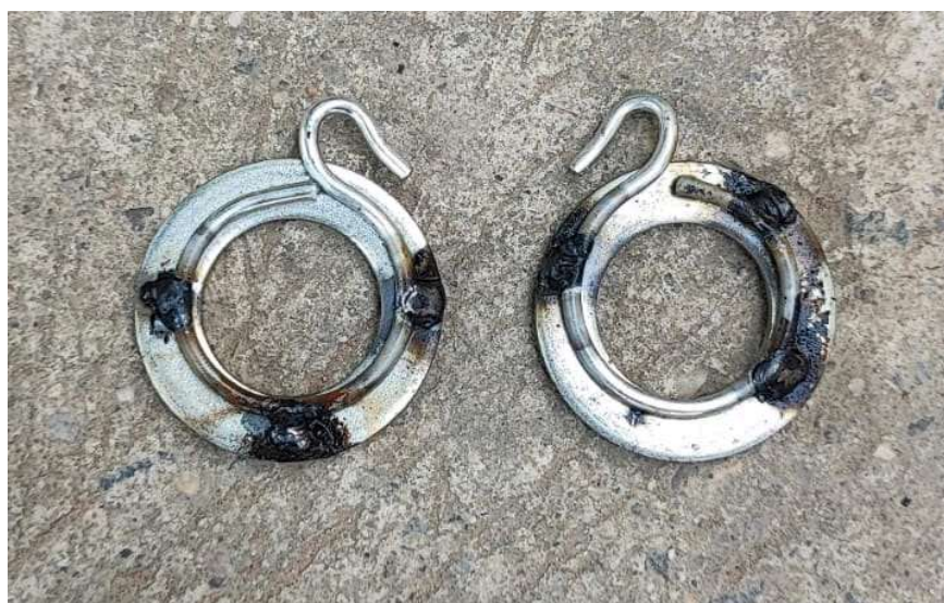
Fig 37.7.2-17 : Welding washer to metal curtain rings
