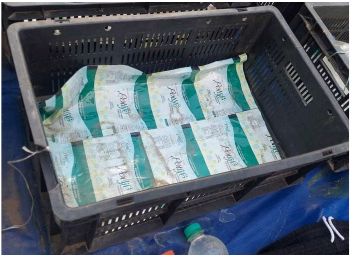
Fig 37.6.3-4 : Placing Of MLP Sheets Inside The Crate
