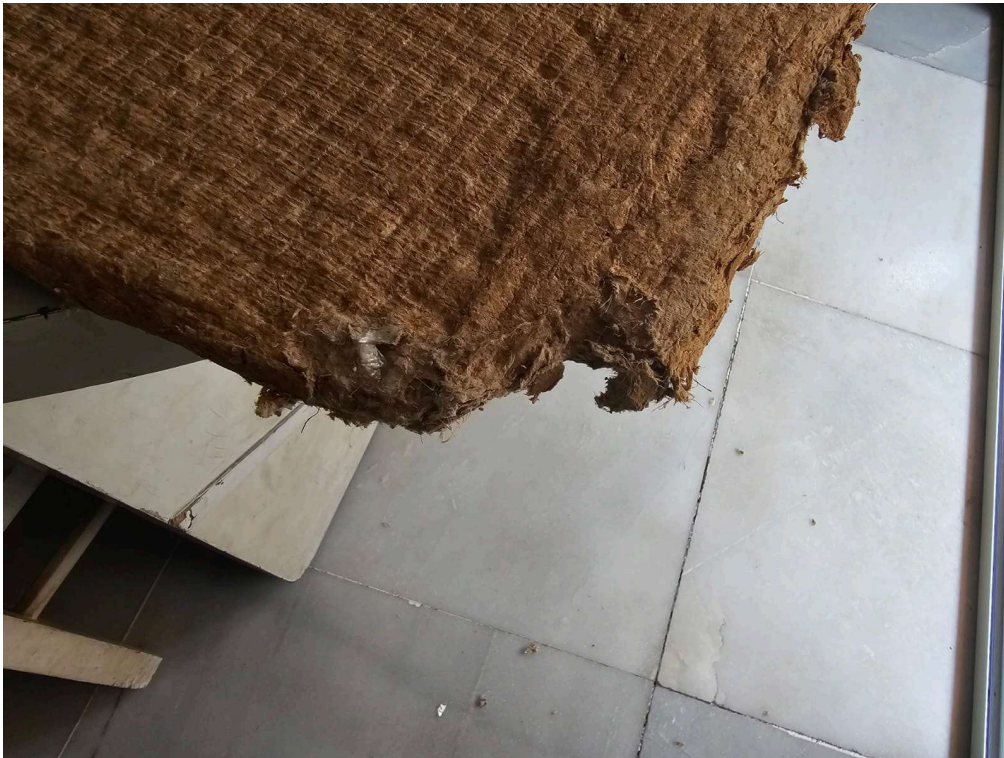
Fig 37.2.3-5 : Check if corners are intact (not broken/chipped)
