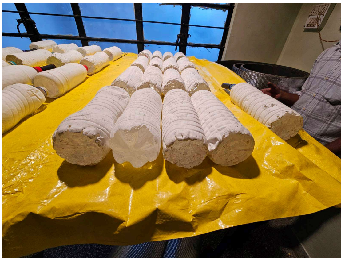
Fig 35.1.1-3 : PET Bottles with Prakritik White Natural Paint on Testbed
