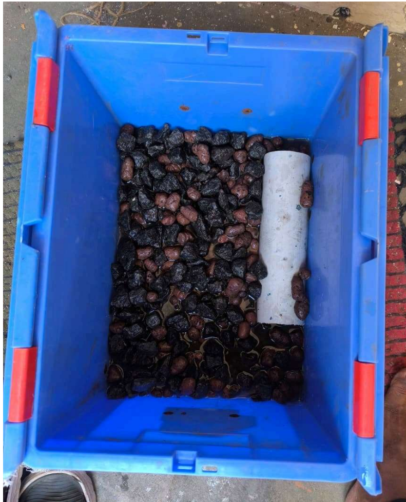
Fig 35.3.4-2 : 20-30 mm LECA Balls Place with Chips, Granules, and Pipe
