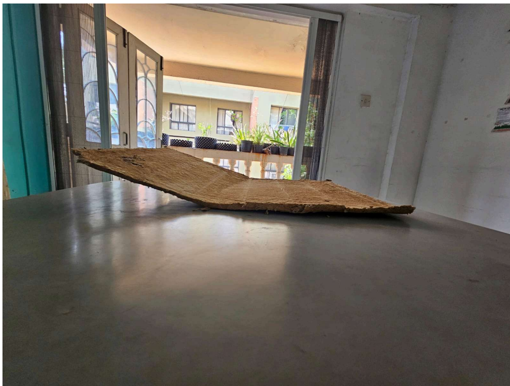
Fig 37.2.3-4 : Check for warping/bending
