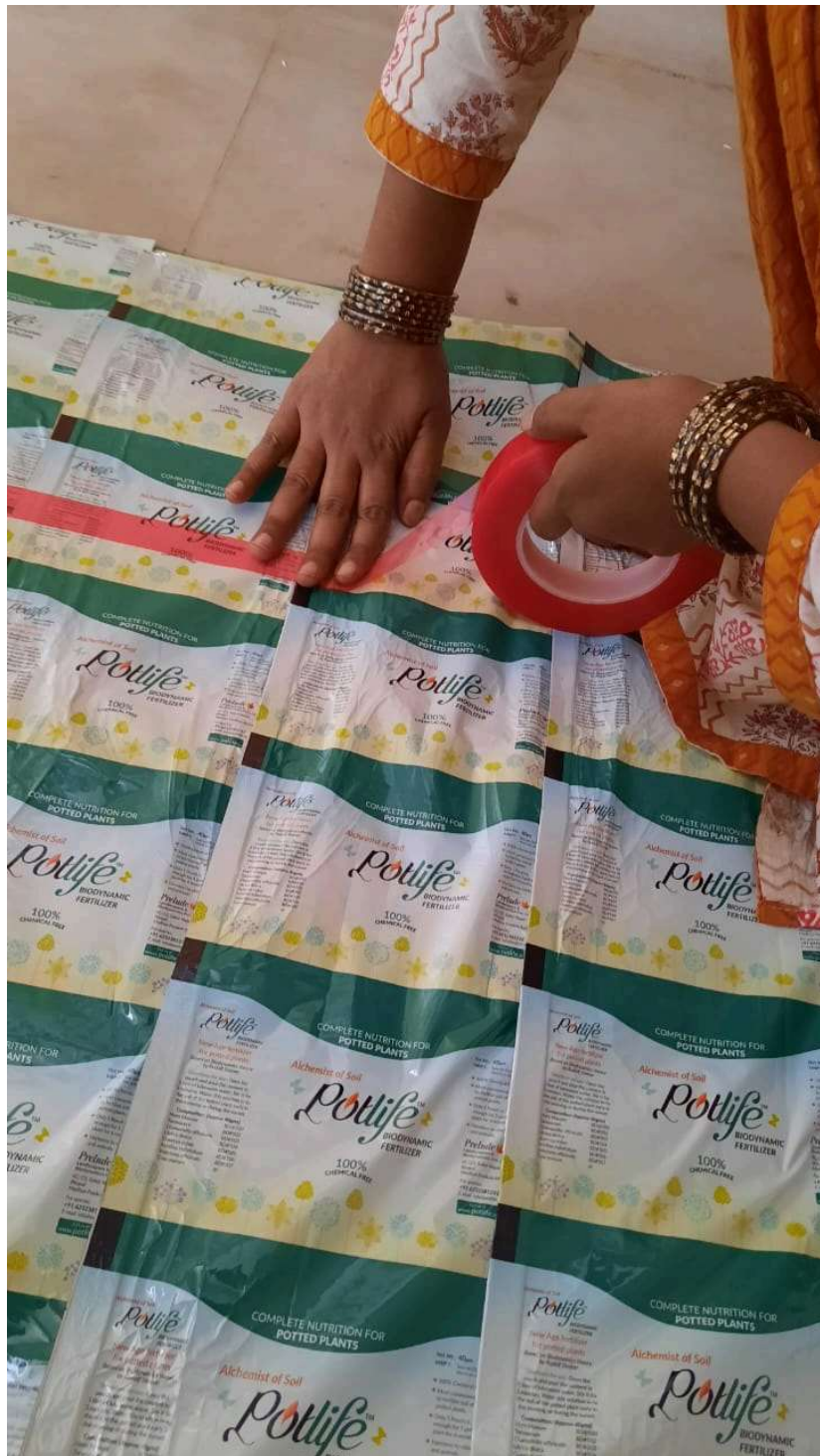
Fig 37.1.2-15 : Placing high strength double side sticky tape for sticking 3 MLP layers
