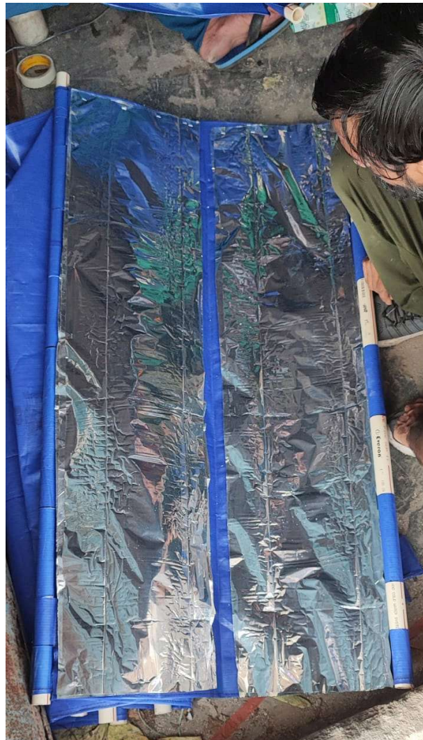
Fig 37.7.2-11 : Attaching MLP to Tarpaulin
