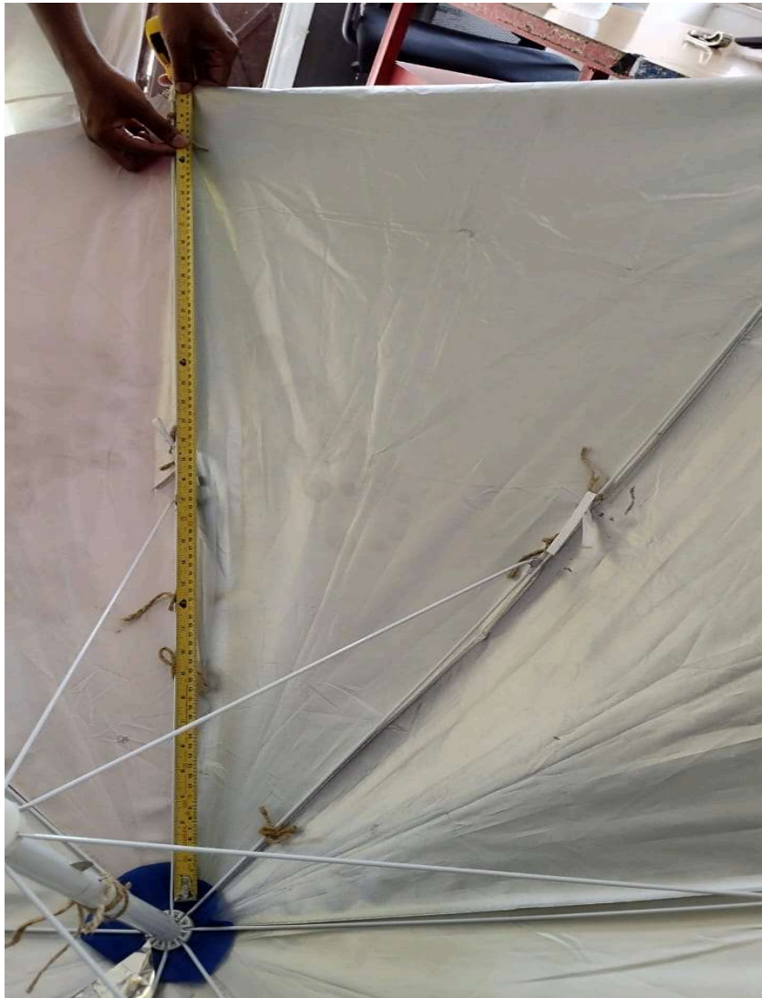
Fig 37.9.2-1 : Measuring the underside of the Umbrella spoke length and segment dimensions
