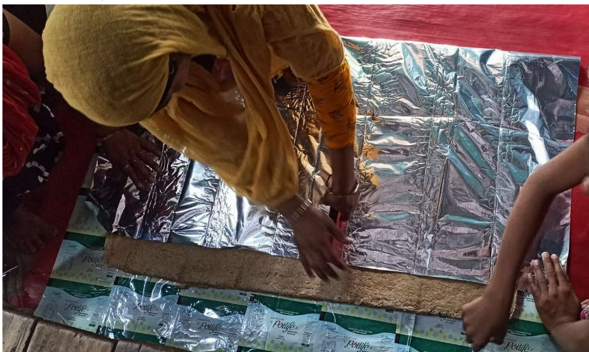
Fig 37.2.4-1 : Wrap the panel with shiny surface facing outside and staple it
