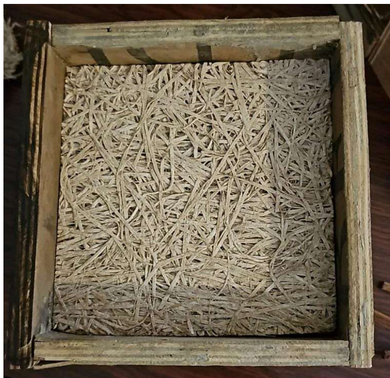
Fig 35.7.1-2 : Wood Wool Panel Testbed (Top View without GI Sheet Covering)
