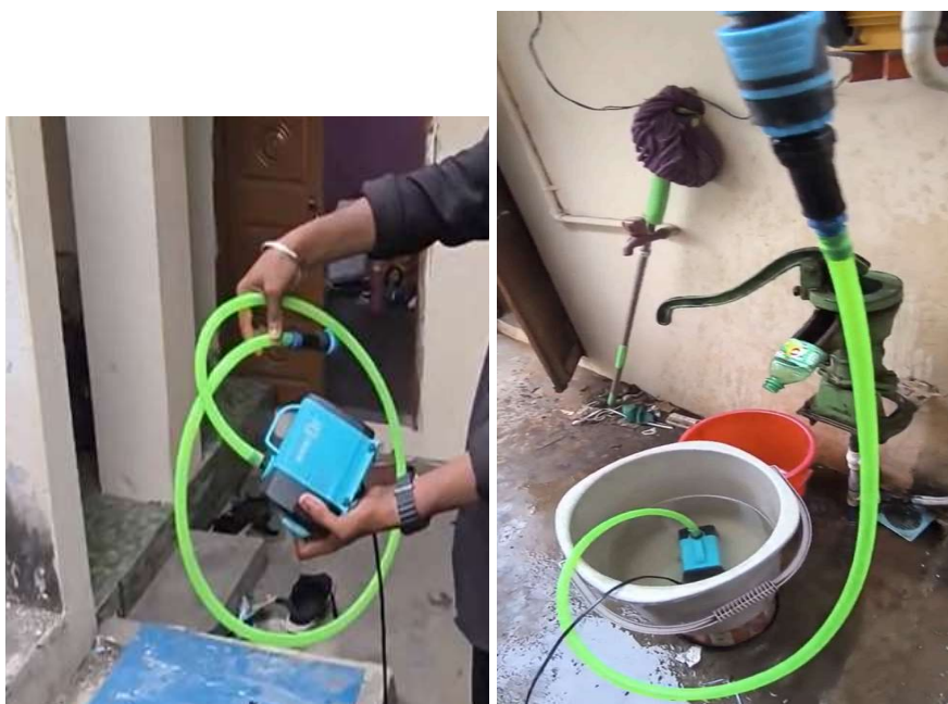
Fig 35.3.2-4 : Submersible Pump Connected with Hosepipe
