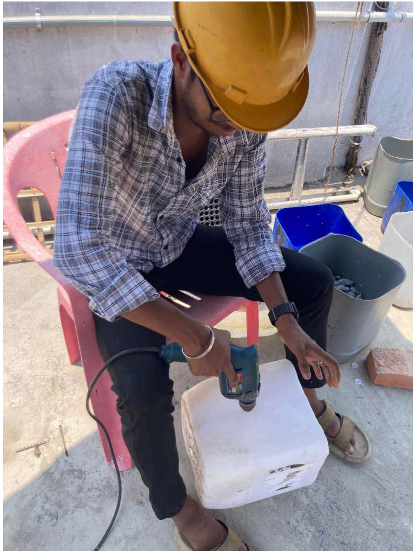
Fig 37.4.2-5 : Drainage hole making on pot
