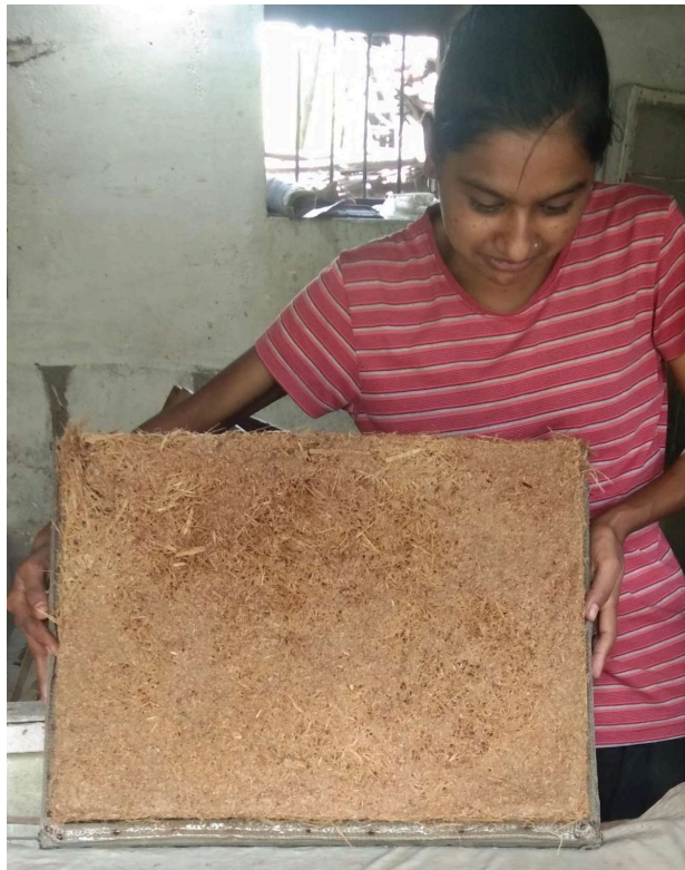
Fig 37.2.2-10 : Lay out the fibres in a wooden mould within a water tank
