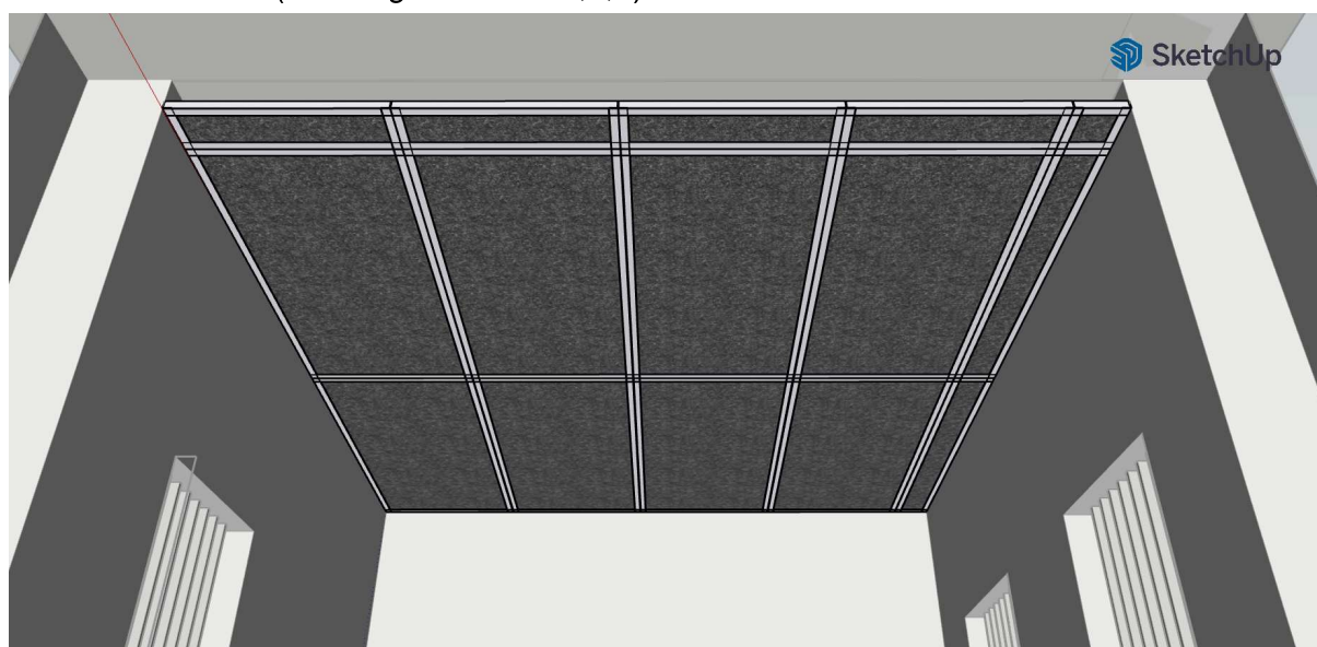
Fig 37.3.2-4 : Metal support framework with panels in place
