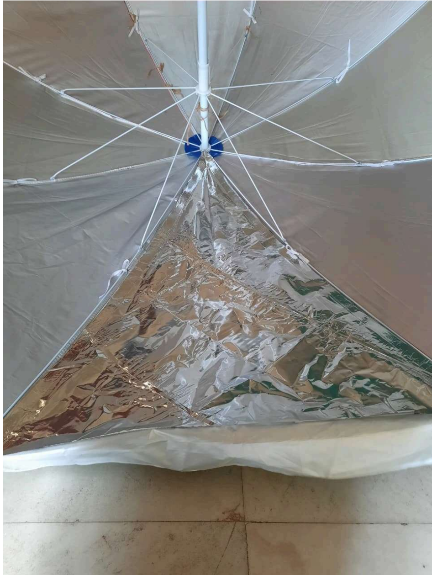
Fig 35.8.1-8 : Triangular Panels Attached to Umbrella Underside
