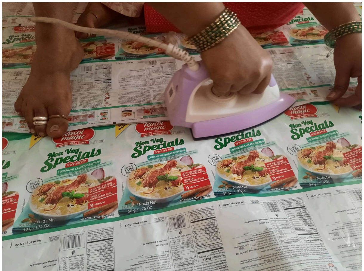
Fig 37.1.2-9 : MLP Sticking using Iron
