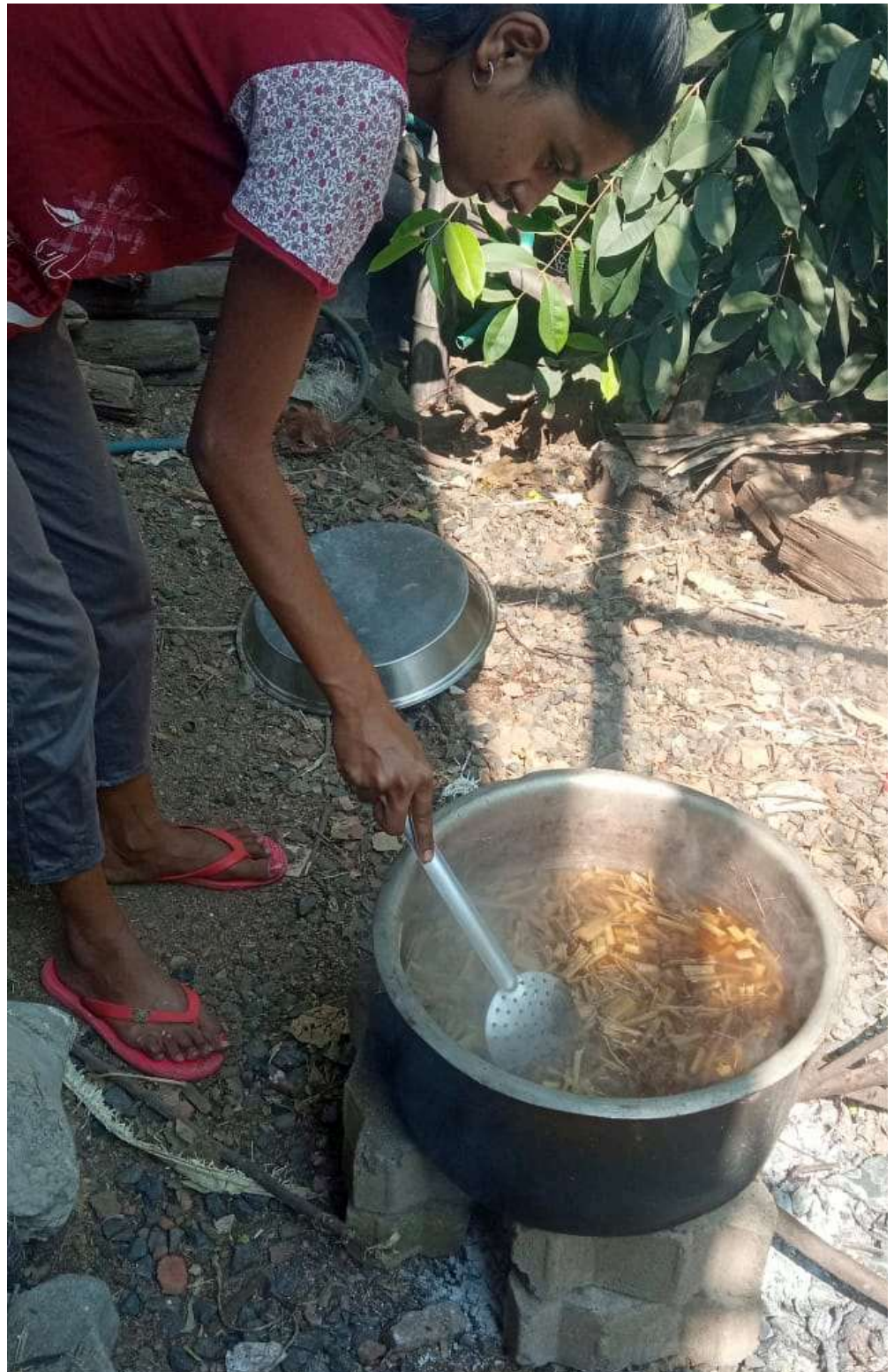
Fig 37.2.2-8: Boil the fibre pieces in sodium carbonate (soda ash)
