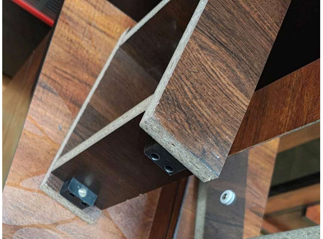
Fig 37.7.2-1 : Wooden shuttering with GD clamp
