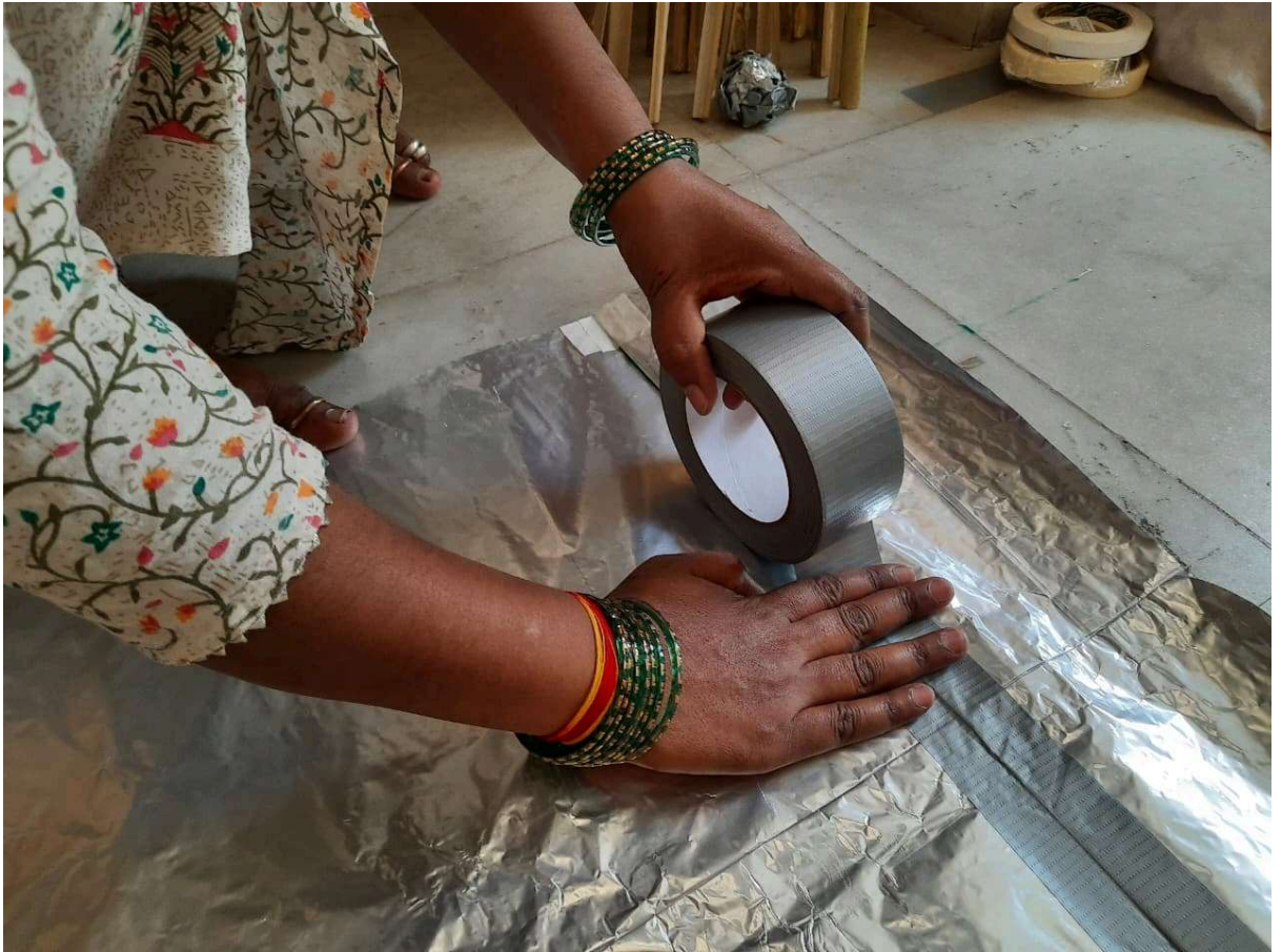
Fig 37.1.2-12 : Placing paper tape for marking 3 inch loop
