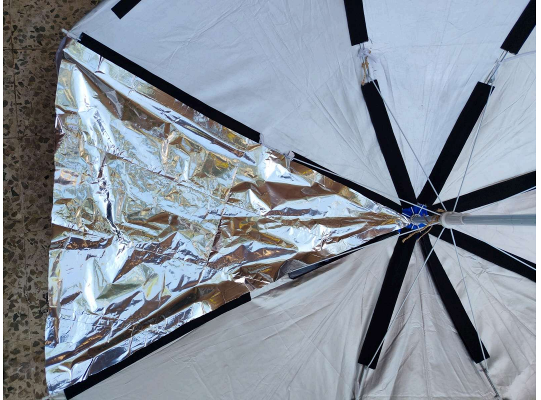
Fig 35.8.1-12 : MLP Sheets Pressed to the Umbrella
