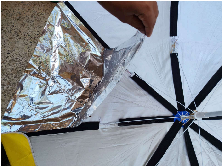
Fig 35.8.1-11 : MLP sheets Bonded Together
