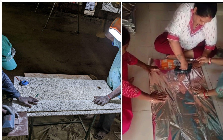
Fig 1: MLP Wrapped Wood Wool Panels
